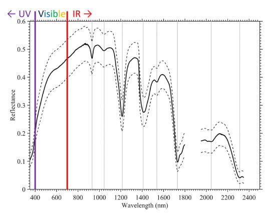
The figure above is an example of a spectral reflectance measurement of marine microplastic particles, showing dips (troughs) of the curve highlighted with gray lines. These dips, called *absorption features*, are unique to the object and can help identify the type of plastic. Dashed lines represent standard deviation.
